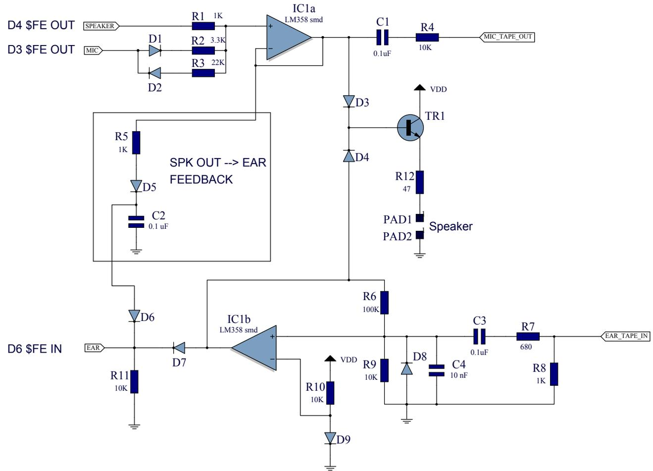
ZX-Spectrum compatible Tape Interface for FPGA zx-badaloc
